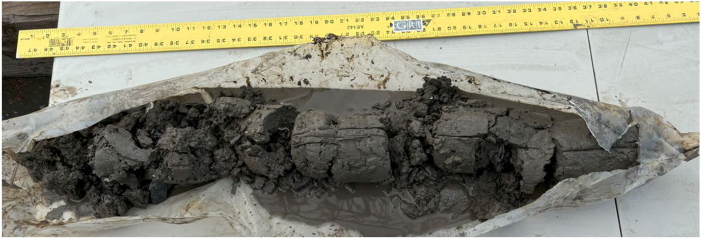
6801-B: BORING 4-A: CORE RUN1 (ELEVATION -14.8 FEET TO -19.8 FEET)
