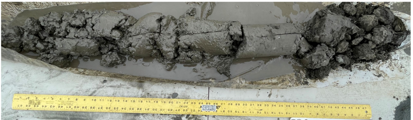
6801-B: BORING 5-B: CORE RUN 2 (ELEVATION -27.6 FEET TO -32.6 FEET)
