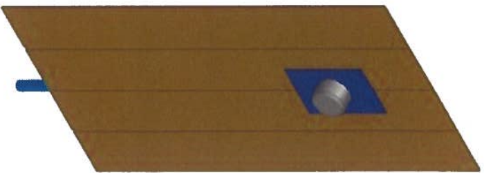
Figure D-1b: Flush- mounted meter base installation
