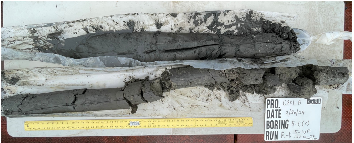
6801-B: BORING 5-C: CORE RUN 1 (ELEVATION -22 FEET TO -27 FEET)
