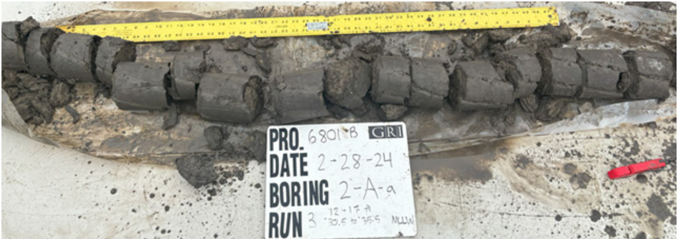
BORING 2-A: CORE RUN 3 (ELEVATION -30.5 FEET TO -35.5 FEET)
