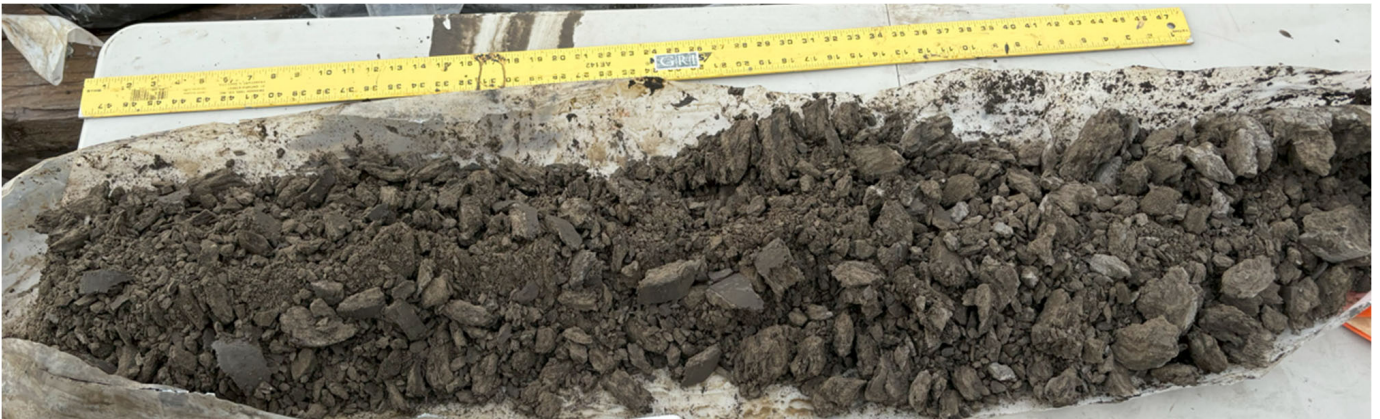
6801-B: BORING 4-A: CORE RUN 2 (ELEVATION -21.3 FEET TO -26.3 FEET)
