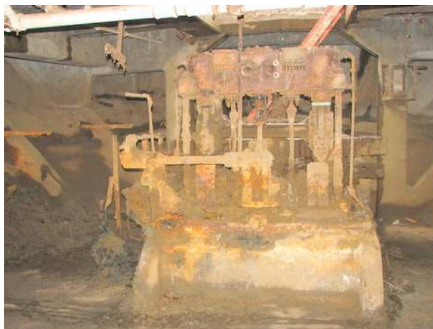
Below decks on the Pasley 1943 steering gear and twin cylinder, vertical reciprocating steam engine
